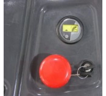
Emergency shut off switch and battery level indicator
